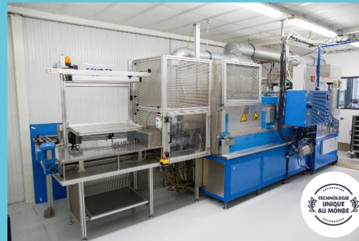
Thermal Toughening of Tubes
